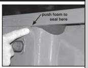
cavity until it fills small opening. Then pull back slightly to fill large cavity.
