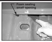
a) At rear of box, spray with b) Compress foam and push c) Push until leading end fills small opening nearest tailgate.
