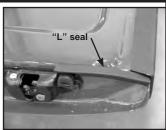
like above at both sides of tailgate. Apply firm pressure to adhesive on both seals.
