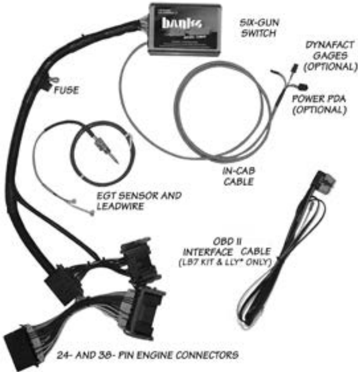
Figure 1 Six-Gun and supplied wiring harness
