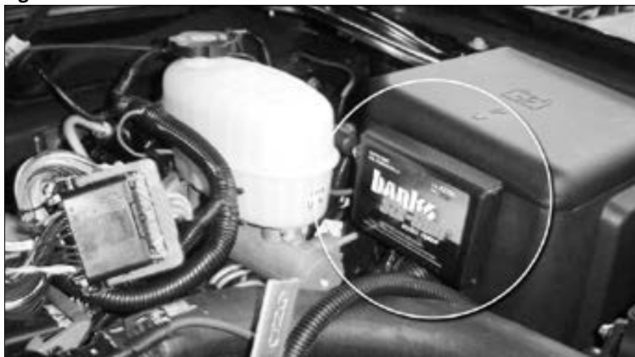
Figure 4 Six-Gun module mounted on fusebox
