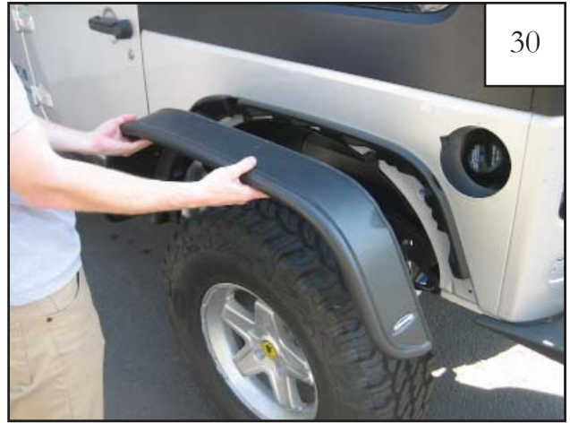
Place the outer flare over the inner pieces and push until snug against the vehicle surface. Make sure splash shield is tucked behind flare.
