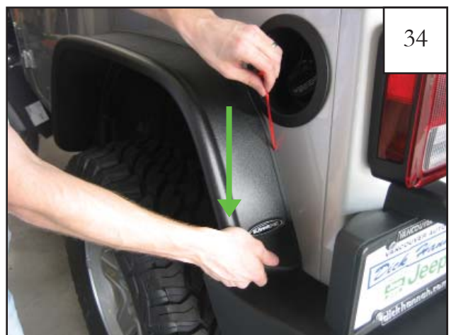
Peel outer tape liner from the double-taped edge trim. Push down lightly on the fender flare to create a small gap between the sheet metal and the edge trim. This makes it easier to pull the red liner.
