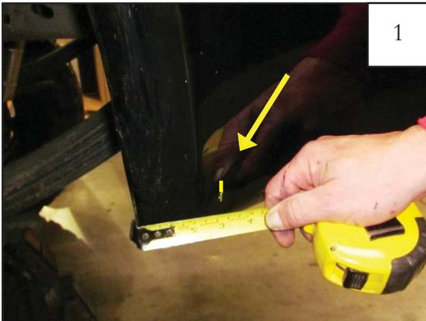
Measure 3" from back side of rear wheel well and mark using a grease pencil.
