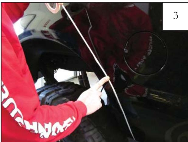
Using marks as a guide, use masking tape to create an arc from the lower mark to the upper mark, then continue around wheel well along style line.
