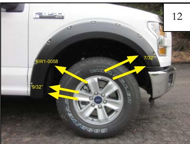
Still holding flare to fender, re-install remaining factory screws removed in Step 4 using 7/32" and 9/32" sockets and wrench. Using a phillips screwdriver, install supplied screw (SW1-0058) into Clip (CL1-0009). Tighten all screws.
