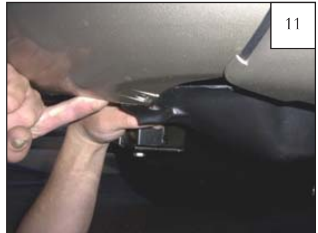
Pull down bumper cover and splash shield.
