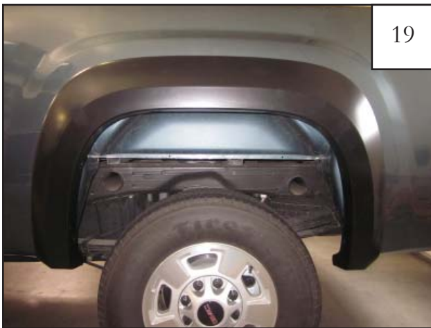
Completed rear flare installation.
