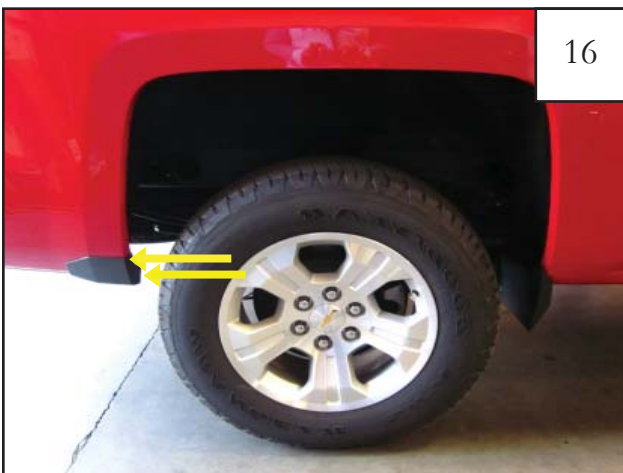
Using a T-15 Torx bit socket wrench, remove factory installed screws from factory rear mudguard. Discard screws.
