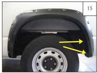
Start two factory screws using an 8mm socket wrench. *Do not tighten.*
