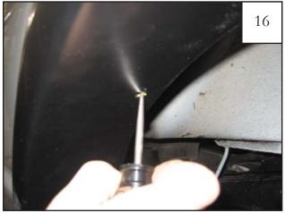
Using an awl or other similar pointed tool make sure that three Clips (CL1-0005) are lined up with the flare holes.
