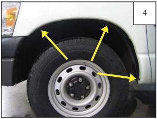
Remove three factory installed screws with 8mm socket wrench. Keep screws for installation of the front flare.
