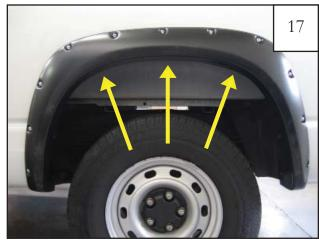
Start three Screws (SW1-0050) through holes in flare and into Clips (CL1-0005) using a #2 Phillips screw driver. *Do not tighten*.
