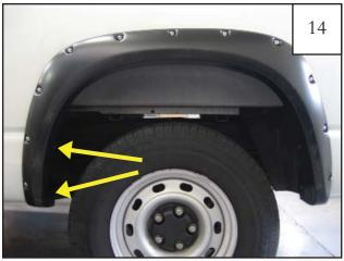
Hold flare in place on vehicle and start Screws (SW1-0056) through holes in flare, Clips (CL1-0011), and into factory holes using a #2 Phillips screw driver. *Do not tighten*.
