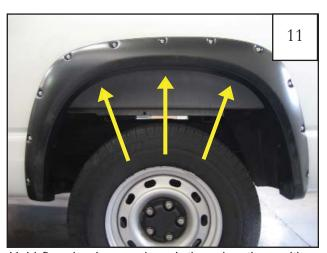
Hold flare in place and mark three locations with a grease pencil using the holes in the flare as a guide. See step 12 & 13.
