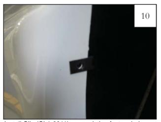
Install Clip (CL1-0011) over existing factory hole.
