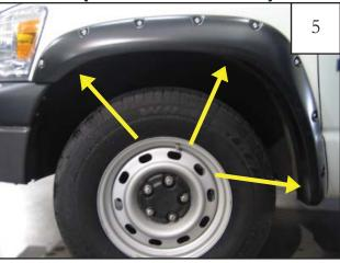
Hold flare to vehicle and reinstall three factory screws with 8mm socket wrench.
