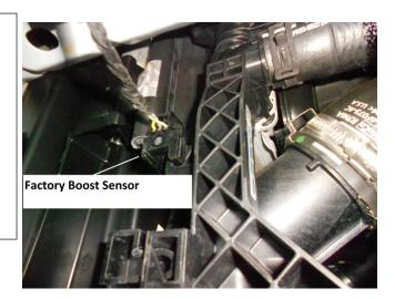
5. Carefully unplug the sensor. \*\*There is a locking tab located at the top of the sensor, squeeze the tab and pull the plug to remove.\*\*
