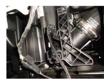
7. Secure the module onto a factory hole on the inner fender core support using the supplied plastic tie as shown in photo.
