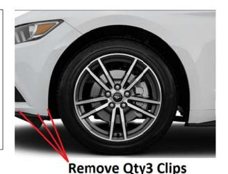
3. Carefully pry clips with a flat blade screwdriver and remove.
