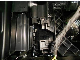
6. Connect the male connector on the Delta Boost module into the factory sensor. Connect the female connector on the Delta Boost module with the connector on the factory harness
