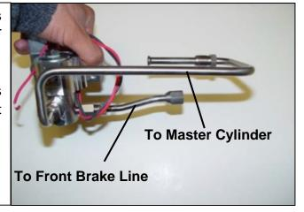
5. Remove left Master Cylinder nut from Master Cylinder.
