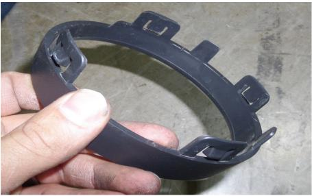
Using a Dremel® tool, cut out sections from the factory fog light housing to remove material and make room for your new Rigid Industries D-Series Fog Lights.
