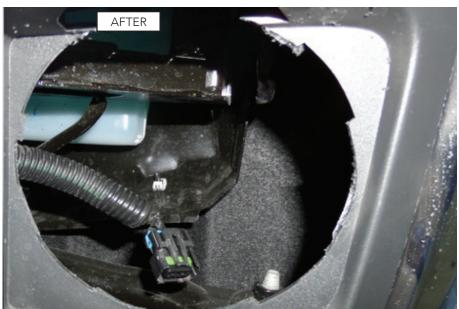
Using your new Rigid Industries Fog Light Bezel as a template, mark the four holes with a pencil that need to be drilled out in order to mount the bracket in the original OEM slot.
