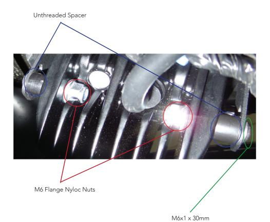
Use 4 Socket Button Head Screws, 4 Washers, and 4 Nyloc Nuts to mount the new Bezel (with your D-Series light attached) into the original OEM fog light slot.
