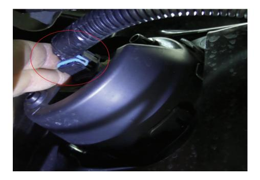
There are 3 fog light retaining clips on the back of the fog light that need to be disconnected. We recommend using needle nose pliers to pinch the connectors and release them.
