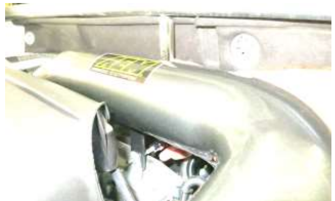
e. Reinstall the tube mounting bolt taking care to position your new intake tube with clearance all around. Tighten both tube mounting bolts.
