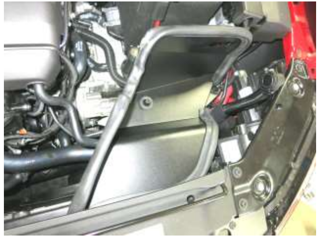
a. Assemble the heat shield according to the diagram on pg2 and install with rubber mount. Lube grommets with glass cleaner if needed to squeeze grommets onto posts.
