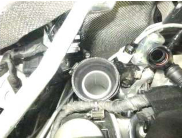
b. Install the turbo-end coupler and both corresponding hose clamps onto the turbo.
