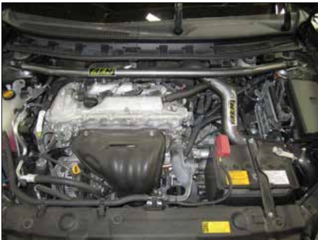
c. AEM Strut Bar installed.
