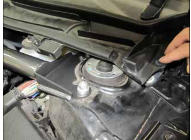
b. Reinstall the plastic clip and 10mm bolt to fasten down the upper plastic fascia.
