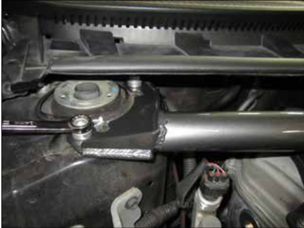
a. Use the two 14mm nuts previously removed to secure the AEM strut bar as shown.
