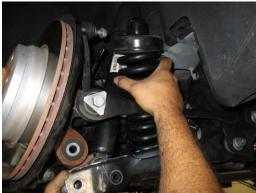
1. Install the factory upper spring seat, onto the new coil spring. Correct orientation would have the part number right side up. Raise the coil into the vehicle, positioning the upper seat into the hole in the chassis.
