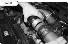
Install 1/8" NPT plugs to back of manifold. Tighten using 3/16" allen key. Install new aFe BladeRunner manifold to vehicle. See notes 2 & 3.
