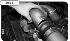
Remove stock manifold out of vehicle.
