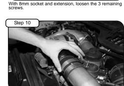
Slide back clamp. Do not tighten.
