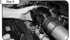
Carefully guide manifold into coupler hose.
