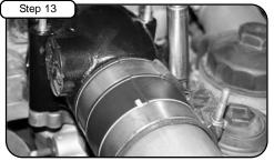
Tighten the clamp using 7/16" socket. See notes 2 & 4
