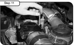
Apply threadlocker to all screws. Secure manifold with flat washers and screws.
