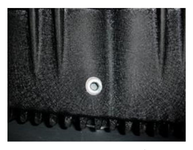
Note: If using a temperature sensor, install it instead of the 1/8" NPT plug.
