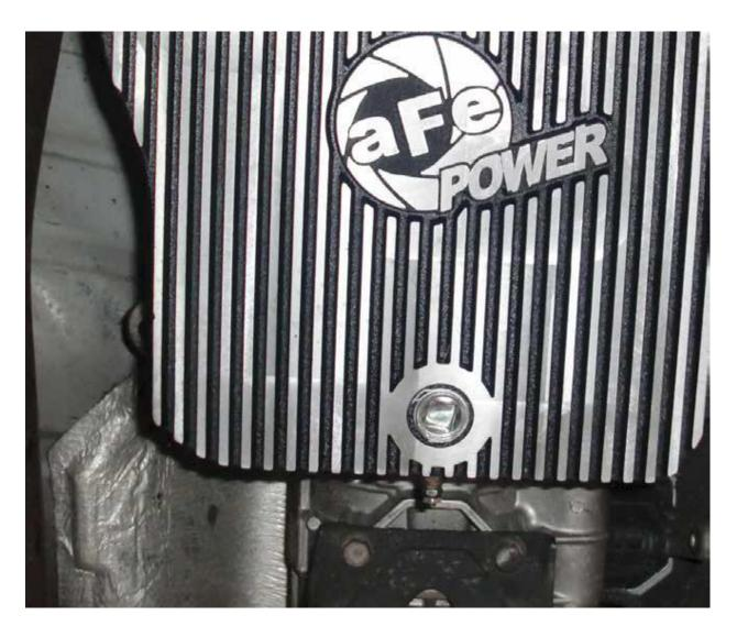
17.Install the supplied 3/4" NPT drain plug on the bottom of the aFe transmission pan.
