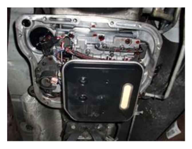
10.Install the supplied transmission filter using the screws removed in step 9.
