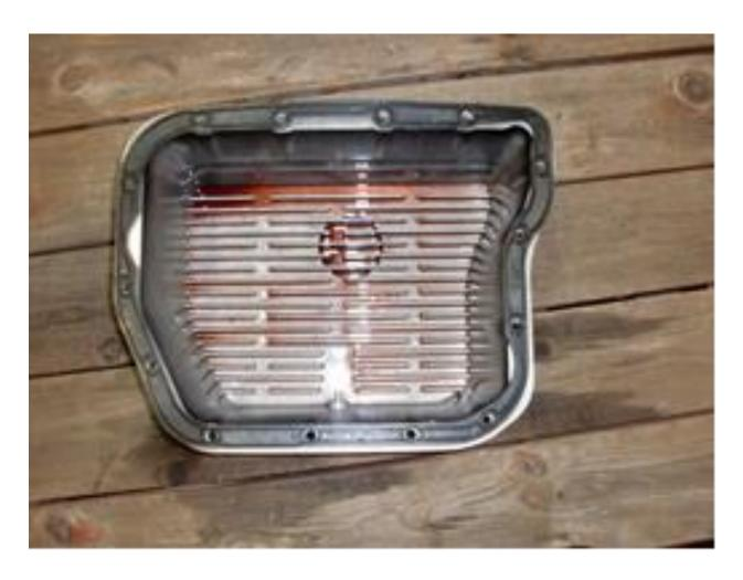
13. Align the supplied transmission pan gasket with the screw holes on the aFe transmission pan.
