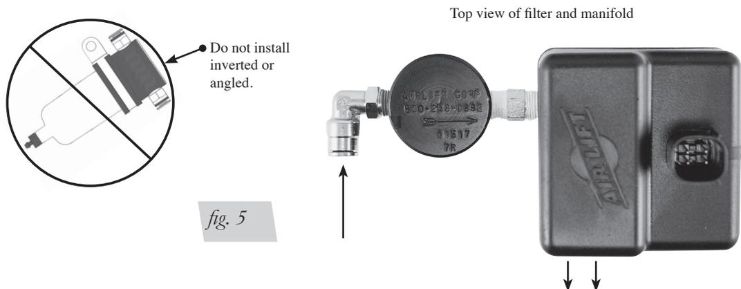
In order to mount the manifold/filter assembly correctly so the filter can drain properly, it may be necessary to rotate the filter on the manifold to orientate it correctly (fig. 1).
