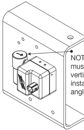
NOTE: Filter must be installed vertically. Do not install inverted or angled!
