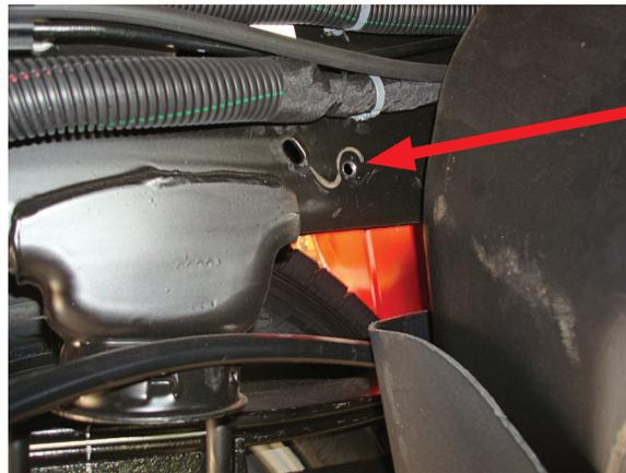
Bolt and retaining bracket removed
