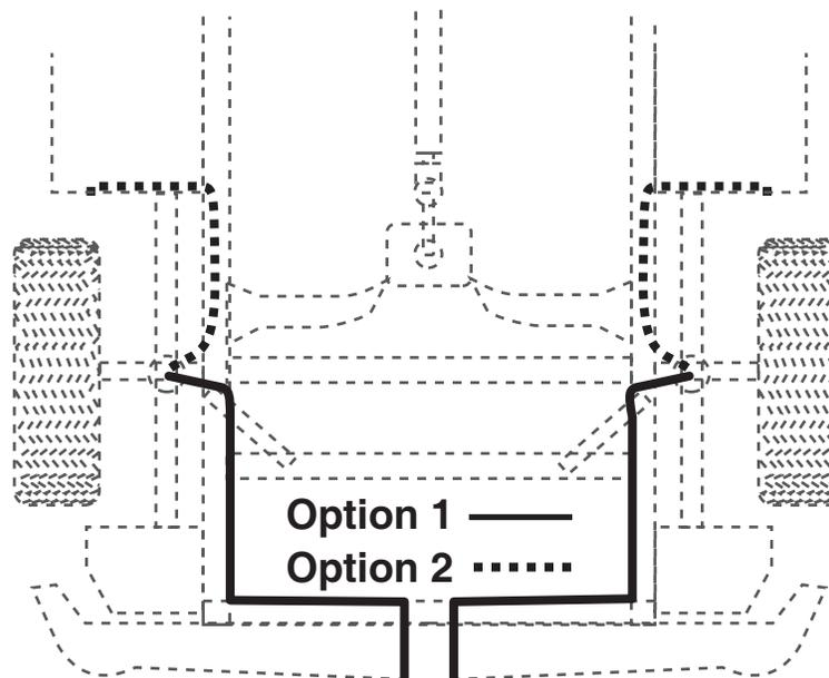
7. Cut off the air line, leaving approximately 12" of extra air line. A clean square cut will ensure against leaks. Insert the air line into the air fitting. This is a push-to-connect fitting. Simply push the air line into the 90° swivel fitting until it bottoms out (9/16" of air line should be in the fitting).
