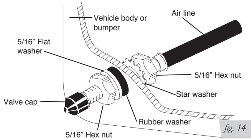
4. Place a 5/16" nut (T) and star washer (V) on the air valve. Leave enough of the inflation valve in front of the nut to extend through the hole and have room for the rubber washer (U), flat washer (N), and 5/16" nut (T) and cap. There should be enough valve exposed after installation — approximately 1/2" — to easily apply a pressure gauge or an air chuck (Fig. 14).
