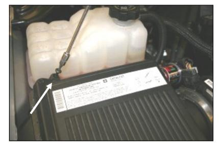
**7.** If you purchased the 200-996 kit, proceed to step # 9. If you purchased a Jr. Kit, remove 4 screws in the factory airbox with a #25 Torx bit, and remove the factory air filter. Proceed to step #8.
