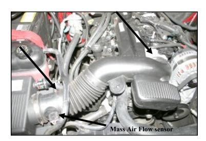
**4.** Loosen two hose clamps on the factory intake tube. One at the throttle body end, and the other at the **M**ass **A**ir **F**low sensor (**MAF**) end.
