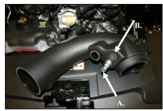
4. Install the Grommets and Fittings into the Airaid intake 5. Using the supplied Torx driver, remove the MAF sen- 6. Install the filter adapter using three 1/4-20 button head tube. A) All models will require the use of the 5/8" Fit- sor from the Factory airbox and create the Tube assemting and the 5/8"Grommet. B) Automatic transmission bly.
