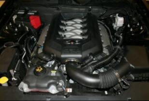
**Disconnect The Negative Battery Terminal! 1.** Remove the Engine cover by simply lifting up, and set aside.
