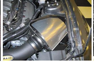
using the 1/4-20 Button Head Screws and Washers. toured edge going away from the filter. Start at the front **NOTE:** Installation of the Rain Shield is optional but of the vehicle and work your way back. Replace the enhighly recommended for vehicles with Power Dome gine cover. hoods with heat extractors.
