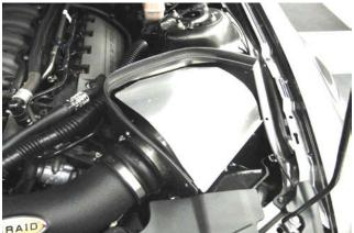
13. Reconnect the Mass Air Flow sensor, which is now 14. Mount the Rain Shield onto the Airbox as shown 15. Install the Weather Strip onto the CAB with the con-
