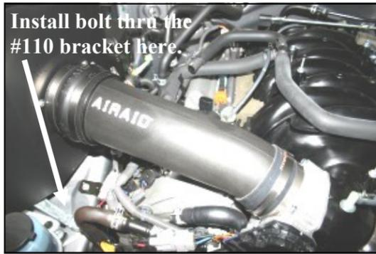
Install bolt thru the #110 bracket here.
