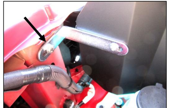
15. Use supplied 10-32 hex head bolt and Fender Washer to secure Panel Bracket. Do not over tighten.
