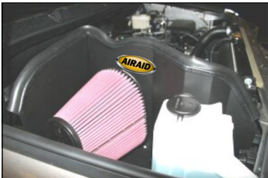
16. Install the Airaid Premium Filter (#1) onto the filter adapter and tighten the clamp. Next install the weather strip (#8) on top of the CAD as shown. For an easier install, start at the fender side of the CAD and work your way towards the radiator. Reinstall the factory beauty cover. Apply the Airaid Decal to the Panel assembly as shown.
