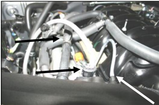
13. Reconnect the MAF wiring harness to the MAF sensor. Reconnect the factory breather hose to the 1/2" barbed coupler using the factory clamp. Reconnect the small vacuum hose to the 3/16" barbed fitting on the Airaid tube.
