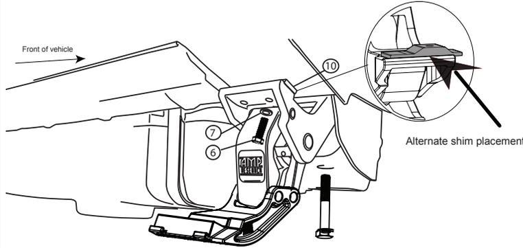
**1** Install Fender Spacer between fender and Idler Linkage (10) Spacer hole and mounting hole faces towards front of vehicle. Install fastener (6) with washer (7), and replace Body mount bolt. Finger tighten only.
