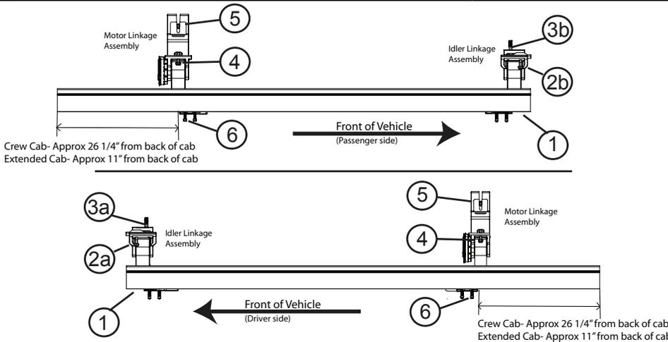
**Note:** Due to vehicle-build variations the Power Step may not correctly align with vehicle cladding. Provided Shims (19) may need to be installed between body mount and idler linkage once Power Step is installed.
