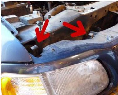
Step 2: Pull up the two locking pins holding in the headlight.
