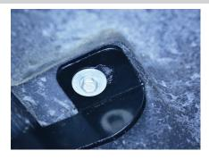
Locate and remove the rear hole plug. Insert an 10mm T-bolt plate into the opening. Slide a plastic bolt retainer over the thread of the bolt to hold the bolt in place.
