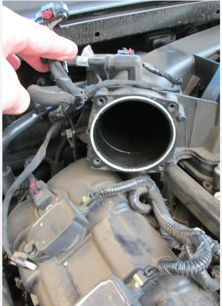
Now with the stock throttle body removed make sure to clean factory o-ring gasket as it will be re-used.
