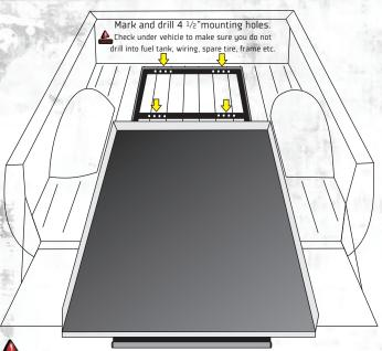
Slowly move upper tray out from closed position and avoid shifting hole placement. Use caution with non-mounted BEDSLIDE.
