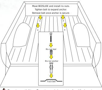
Do not over tighten. Do not use air impact tools with riv nuts.
