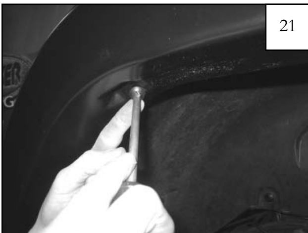
Install supplied Truss Head Screws through holes in wheel well and into #14 U-Clips installed in Step 15 (5 places).
