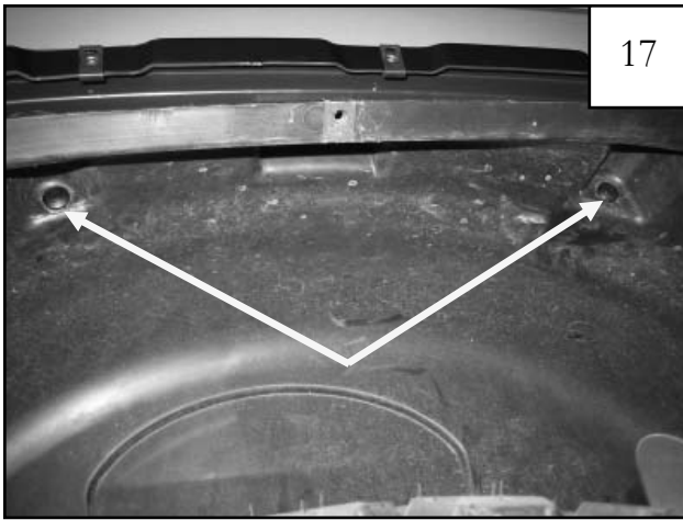
Position splash shield in wheel well, and install two supplied Plastic Phillips Head Tuflocs in upper pockets using a pushing-twisting motion.
