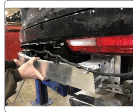
6. Reinstall exhaust bracket, using hardware removed in Step 4. Secure bracket, bumper beam, and hitch to vehicle.
