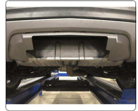
2. Pull back wheel well cover to remove (1) fastener using T-15 socket, on each side of vehicle. Carefully remove lower fascia, starting from outside and moving towards center on each side.
