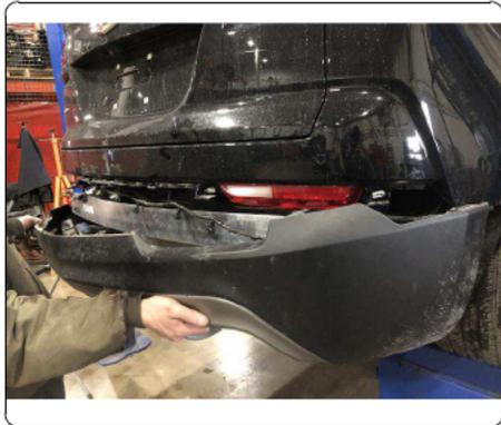
4. Remove bumper beam by locating and removing (4) fasteners on each side using 15mm socket. Unclip exhaust bracket from rear of vehicle to lower exhaust.
