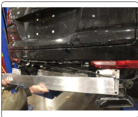
5. Raise hitch into position using vehicle studs to align. Install bumper beam over hitch.
