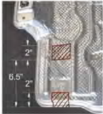
HEAT SHIELD TRIM DIAGRAM
