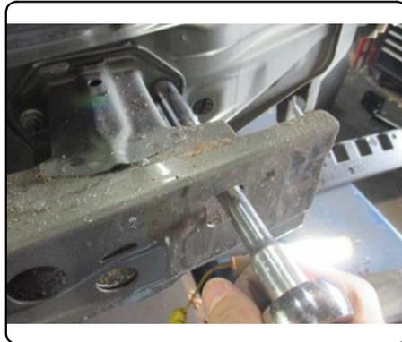
6. Fold the center bumper cover mounting tab flat against the rear bulkhead of the vehicle. Raise the hitch and bumper beam back into position on the studs, center and loosely reinstall the nuts removed in step 5.
