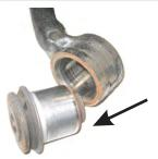
Factory bushing metal shell must be pressed out of upper control arm for Energy Suspension polyurethane bushings to fit properly.
