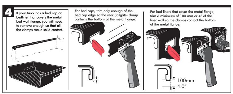
Ensure the clamp is positioned under the bed wall flange. Hand tighten until the clamp makes contact, then tighten an additional two turns. Make sure to secure to the bed wall flange and Not to the lip of the bed liner or rail cap. Do Not use a wrench to tighten.
