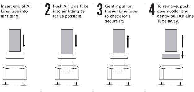
**Removal Tip:** Use a 1/4", 5/16", or 6mm open-ended wrench to push the collar down.
