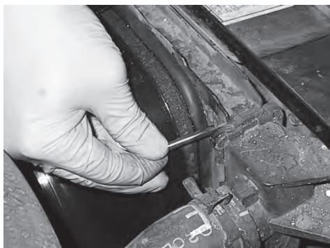
Install temp. probe near inlet hose...
