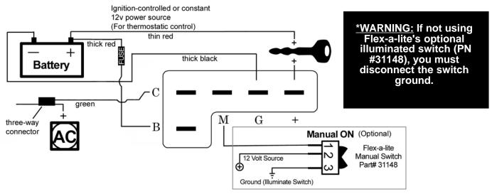
Note: To stop the fan from activating thermostatically, omit the lead to the "+" terminal of the control box. "B", "G", & "M" must remain connected.
