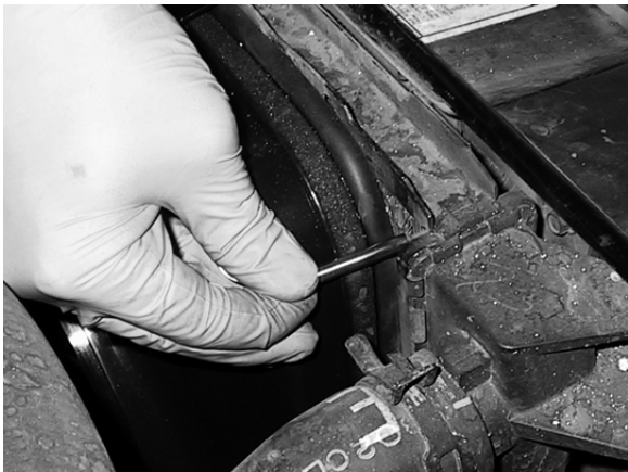
Install temp. probe near inlet hose...
