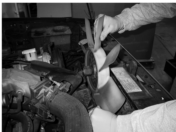
Remove the original fan...
