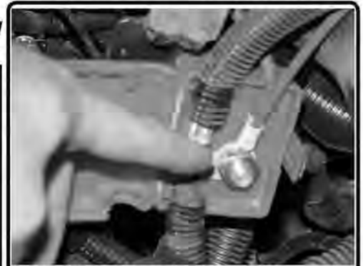
Detail 7- Tap into the junction box near the battery to provide direct battery + power to the VSC.
