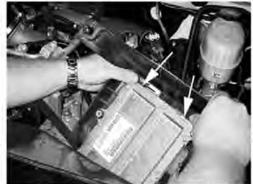
Detail 1- Detach transmission TCM from the cover by un-clipping it. Do not unplug the TCM!
