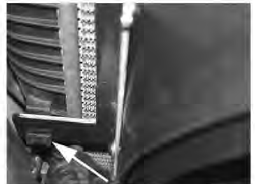
Detail 6 - Lower the fan assembly into place over the radiator core and tuck the bracket "ears" into the pockets on the tanks as shown.
