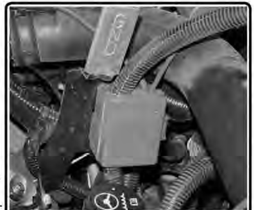
Detail 8- The junction box after installing a power lead for the VSC
