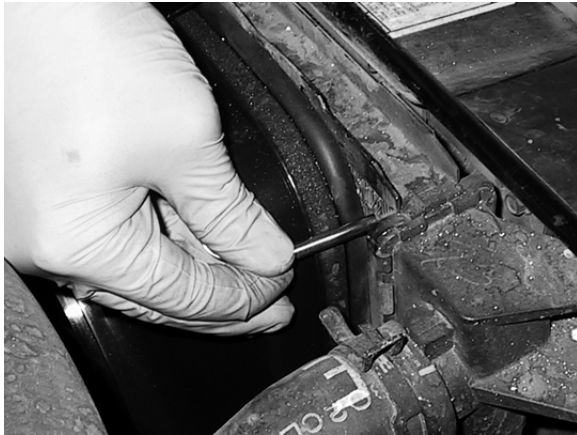
Install temp. probe near inlet hose...
