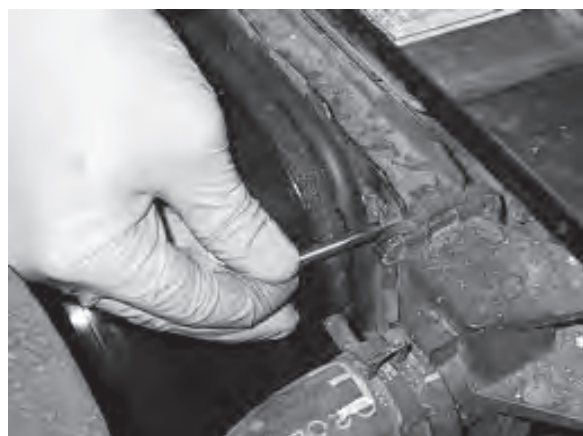
Install temp. probe near inlet hose...
