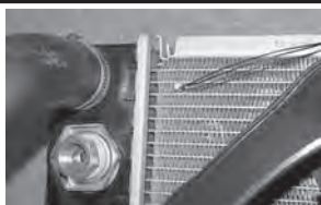
Install the temp. probe near the inlet hose, leaving 1/4" of the probe protruding from the core.
