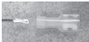
When crimping the temp. probe wires, strip back the insulation, then fold wire back on itself to double thickness
