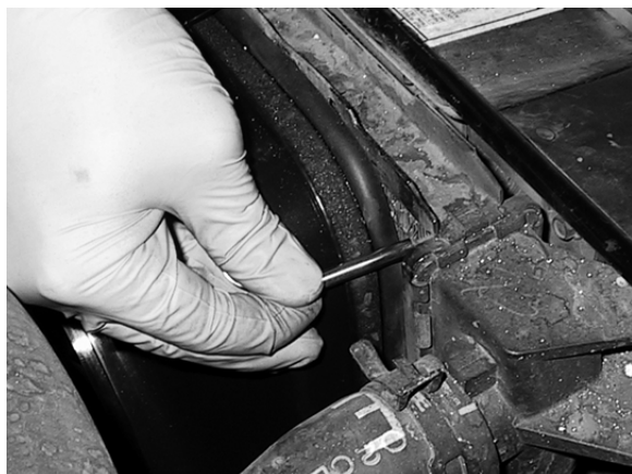
Install temp. probe near inlet hose...
