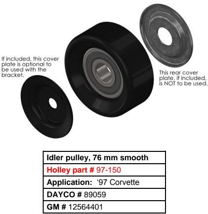
When installing the passenger's side A/C bracket, a smooth pulley will need to be installed on the tensioner assembly. Retain the removed grooved pulley for bracket assembly.
