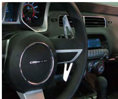
Paddle Shifter Kit 5385430 ("Jagan" paddle Kit) 5385432 (Standard paddle Kit) For Automatic Transmission
