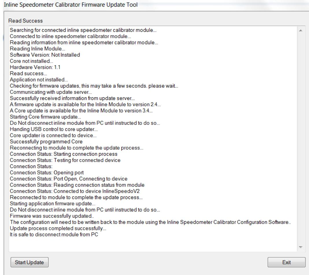
**Once the update is complete, click “Exit” to close out the Update Tool. The module should now be updated to the latest firmware version. To verify, run the Inline Speedometer Corrector Program, and click “Read Device”. The new software version will begin with 03.04.**
