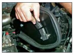
15. Reconnect the air temperature sensor electrical connection as shown.
