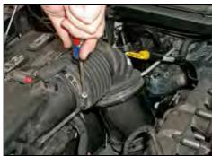
3. Loosen the hose clamps at the turbo inlet and the air box outlet as shown.
