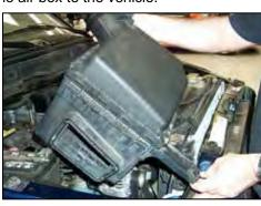
6. Remove the complete air box assembly from the vehicle as shown.
