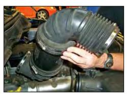
4. Remove the intake tube from the vehicle as
