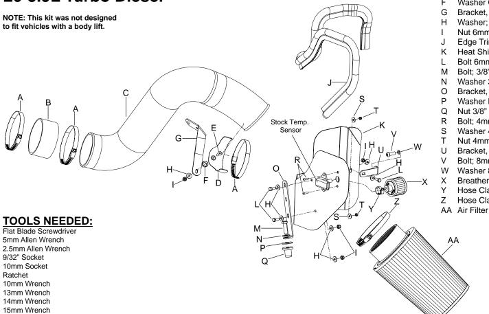
Hose Clamp #64 3 08645 Silicone Hose, 4"ID X 2"L 08761 Intake Tube 087084 Saddle Bracket 078855 Bolt 6mm 08376 Washer Cup 08180 Bracket, Lg. Twist 07160 Washer; .250"ID X .675"OD 08275 Nut 6mm Nylock 07553 Edge Trim 46"L 102487 Heat Shield 07486 Bolt 6mm-1.00 X 16mm 07703 Bolt; 3/8"-16x1.250" 07779 Washer 3/8" Flat 08134 Bracket, Lg. 07159 Washer Fender 08126
