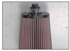
23. Install the grommet and air filter minder that was removed in step 21 onto the  $K\&N^{\scriptsize @}$  air filter as shown.
