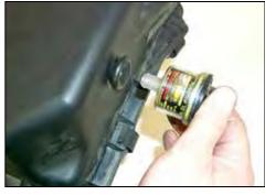
21. Remove the air filter minder and grommet from the stock air box lid as shown.
