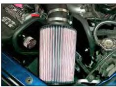
25. Install the  $K\&N^{\otimes}$  air filter onto the intake tube as shown.
