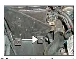
7. Remove the air box mounting grommet as
