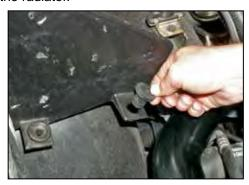
14. Install the nut insert onto the air box mounting tab as shown.
