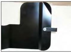
9. Install the short "L" bracket onto the heat shield with the provided hardware.
