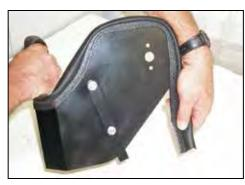
10. Install the edge trim onto the heat shield as shown.
