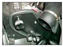
24. Install the  $K\&N^{\scriptsize \$}$  air filter onto the air temperature sensor as shown.
