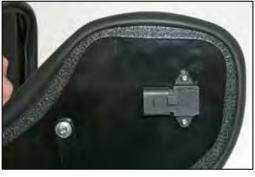
12. Install the temperature sensor onto the heat shield with the provided hardware as shown.
