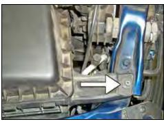
5. Loosen and remove the 10mm nut that retains the air box to the vehicle.
