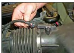
2. Disconnect the air temperature sensor electrical connection.
