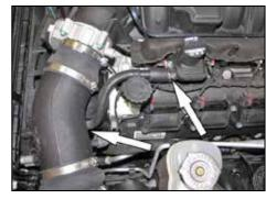
21. Install the assembled vent hose onto the fitting installed in the K&N<sup>®</sup> intake tube and then attach the open end to the valve cover port and secure with the provided hose clamp.
