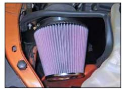
24. Install the K&N<sup>®</sup> air filter and secure with the provided hose clamp. NOTE: Drycharger<sup>®</sup> air filter wrap; part # RF-1042DK is available to purchase separately. To learn more about Drycharger<sup>®</sup> filter wraps or look up color availability please visit http://www.knfilters.com<sup>®</sup>.
