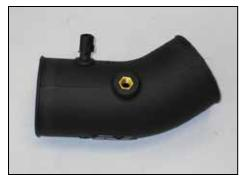
16. Install the provided grommet and the factory inlet air temperature sensor into the  $K\&N^{\mbox{\ensuremath{\mathbb{S}}}}$  intake tube as shown.
