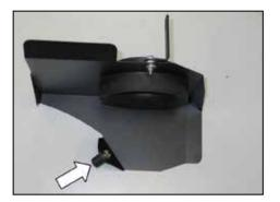
10. Install the provided rubber insert onto the heat shield as shown and secure with the provided hardware.
