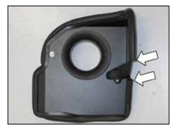
11. Install the provided edge trim onto the heat shield as shown.
