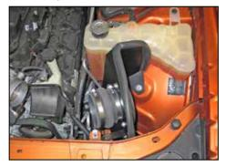
13. Set the heat shield assembly into position in the engine bay so the rubber insert passes into the air box mounting hole in the inner fender. Do not secure the heat shield at this time.
