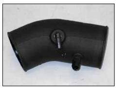
17. Install the provided 90° vent fitting into the  $K\&N^{\circ}$  intake tube as shown.
