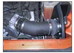
18. Install the K&N<sup>®</sup> intake tube into the silicone hump hose and then into the silicone step hose at the throttle body. Align the intake tube and heat shield for proper fit and then secure the intake tube with the provided hose clamps and the heat shield bracket with the factory air box retaining bolt removed in an earlier step.
