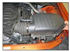
7. Lift up and remove the complete intake track from the vehicle.
