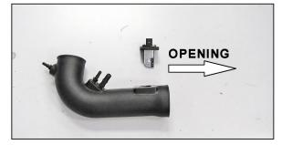
23. Install the mass air sensor assembly into the K&N<sup>®</sup> intake tube so that the opening in the sensor faces towards the filter end of the tube and secure with the provided hardware
