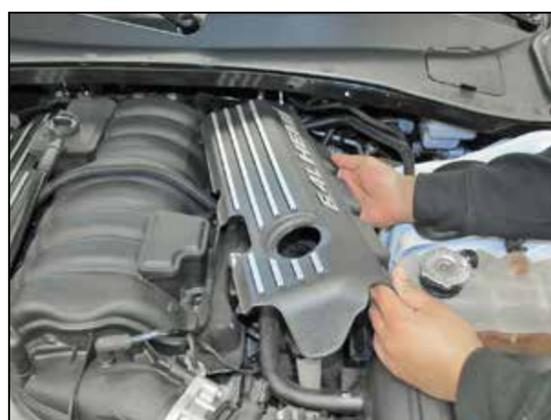
3. Lift up and remove the driver side ignition coil cover as shown.
